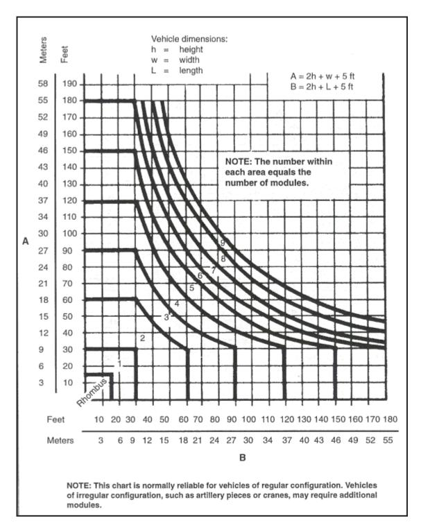
Figure C-2. Module determination chart.
