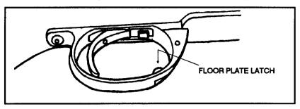
Figure 2-17. Floor plate latch.
