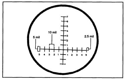
Figure 4-19. M19 mil-scale reticle.
