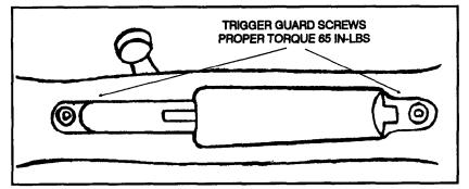
Figure 2-15. Trigger guard screws.
