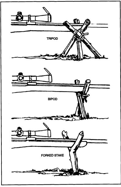
Figure 3-12. Field-expedient tripod, bipod, and forked stake.
