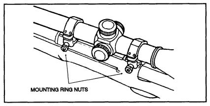
Figure 2-14. Mounting ring nuts.
