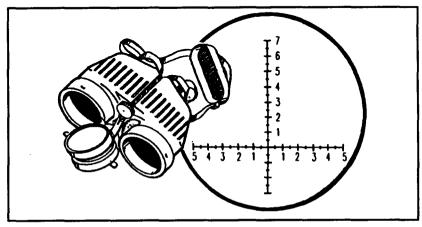
Figure 2-33. M22 binoculars and reticle.
