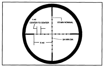
Figure 4-20. M3A mil-scale reticle.
