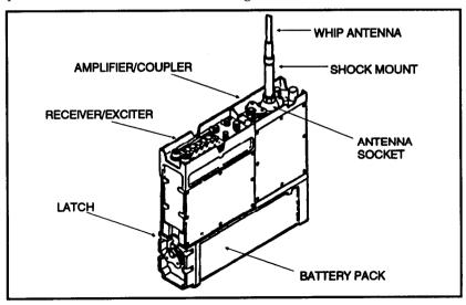
Figure 2-35. AN/PRC-104A radio transceiver.
