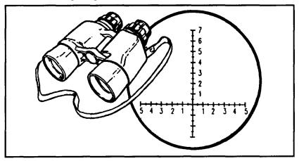
Figure 2-32. M19 binoculars and reticle.
