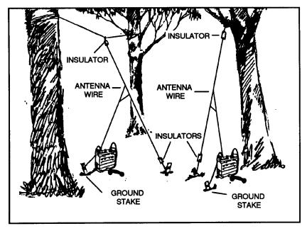
Figure 7-8. Improvised vertical half-wave antenna.
