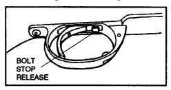
Figure 2-4. Bolt stop release.
