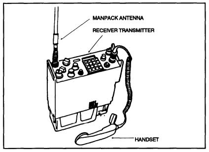
Figure 2-36. AN/PRC-119 radio.
