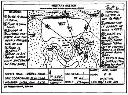
Figure 4-23. Example of completed DA Form 5788-R for topographic sketch.
