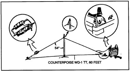
Figure 7-9. Verticle half-rhombic antenna.
