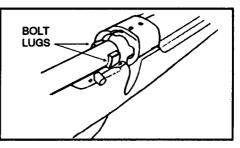
Figure 2-5. Bolt alignment.
