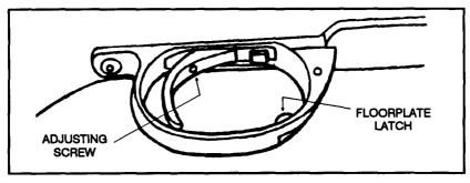
Figure 2-6. Trigger adjustment.
