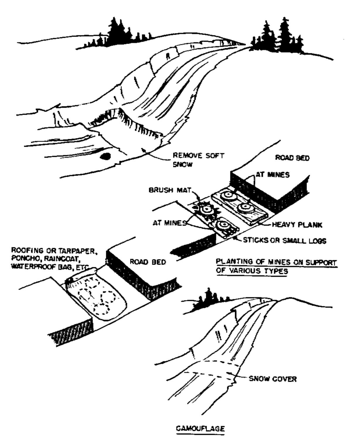
Figure 6-32. Laying mines in deep snow.
