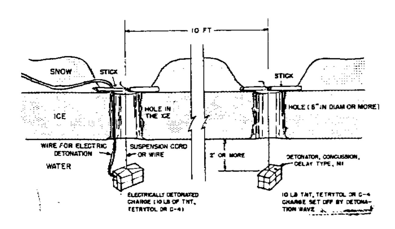
Figure 6-34. Method of placing charges in ice.
