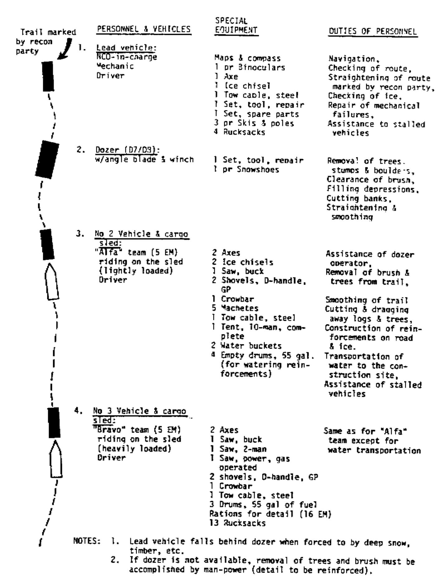
Figure 5-6. Construction detail for winter roads.
