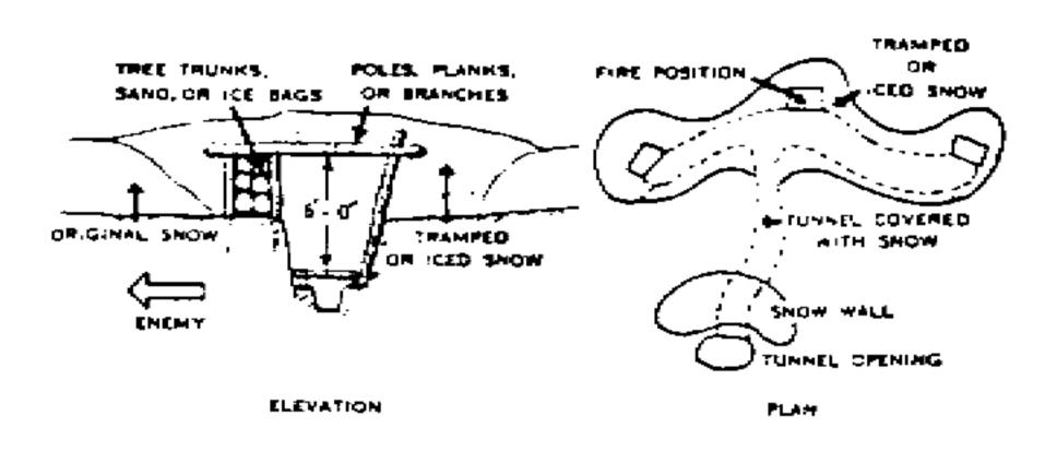
Figure 6-1. Example of position constructed in snow and extended into frozen ground.
