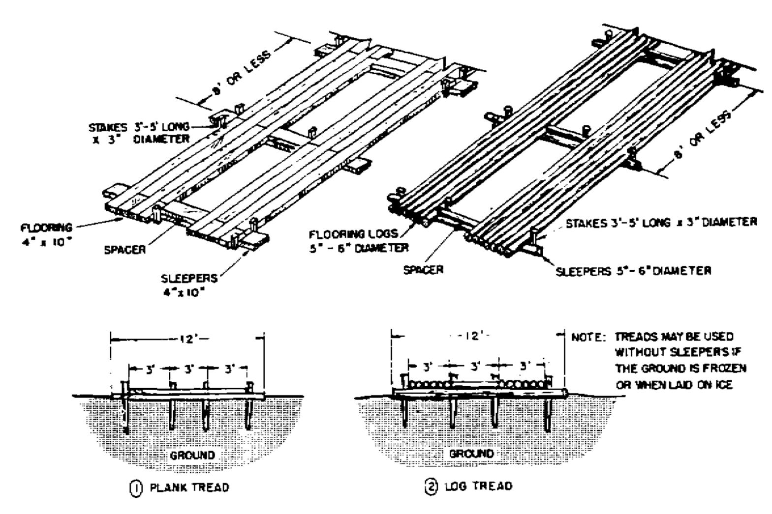
Figure 5-10. Road reinforced with tread.
