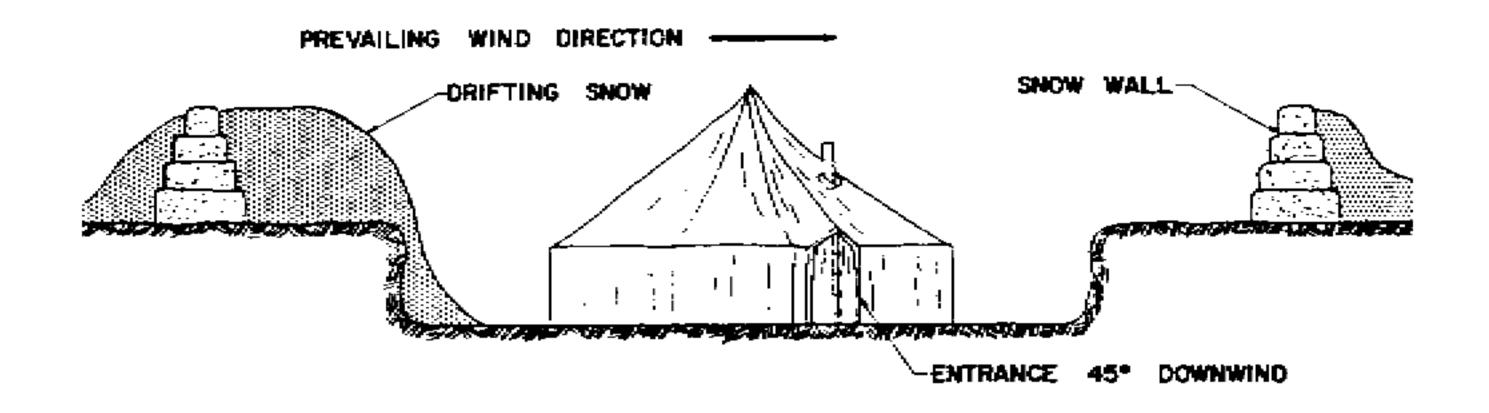
Figure 3-5. A tent dug in with snow wall windbreak.
