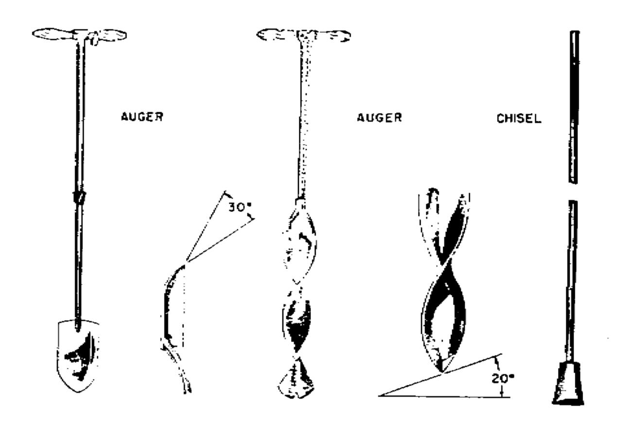
Figure 6-35. Types of ice augers and ice chisel.
