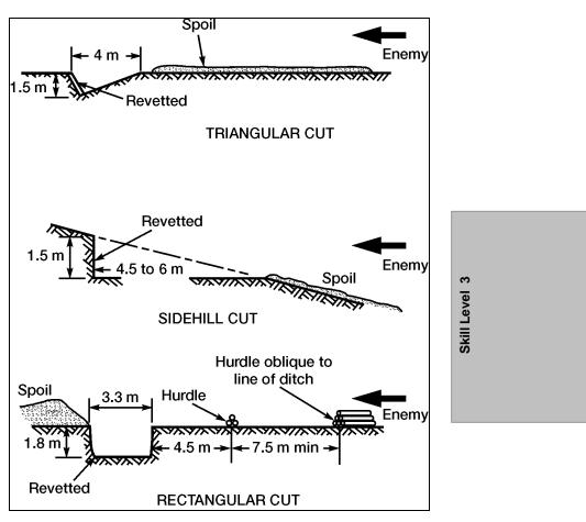
Figure 052-195-3066-12. Tank Ditches
