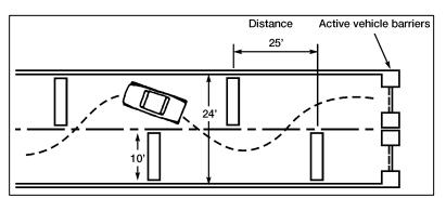
Figure 052-195-3066-16. Concrete Obstacle Placement
