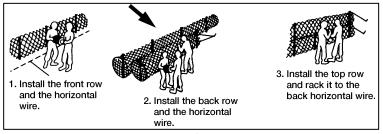
Figure 052-195-3066-3. Install Concertina and Horizontal Wire
