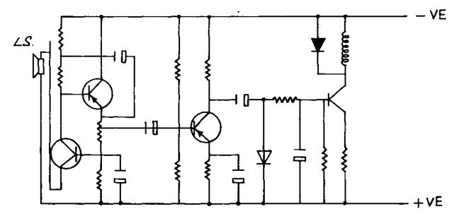
FIG. 79 ACOUSTIC SWITCH
