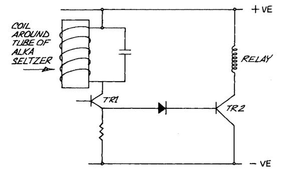
FIG. 74 ALKA SELTZER ELECTRONIC DELAY
