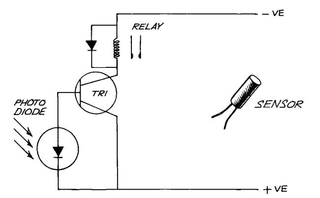
FIG. 82 INFRA-RED SENSITIVE SWITCH
