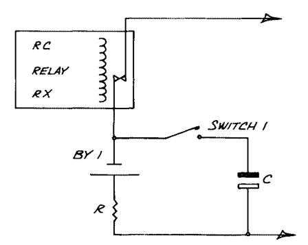
FIG. 72 ELECTRONIC DELAYED ARMING
