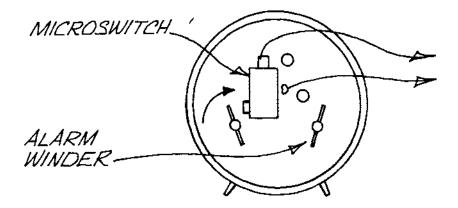
FIG. 59 ALARM WINDER & MICROSWITCH
