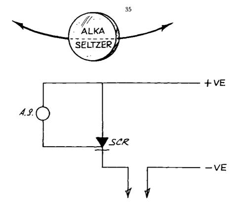
FIG. 86 ALKA SELTZER TABLET SWITCH
