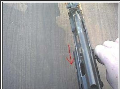
With the spring removed pull the action all the way back, when it reaches the rear of the receiver you should be able to lift up and remove it.
