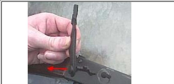
Finish rotating the lever in the same direction until the tab is above the FCG, by now the lever should be able to be removed by guiding the "U" shaped tabbed area out of the receiver through the special designed hole on the right side (ejection port side) of the receiver.
