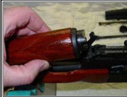
Using an open end or adjustable wrench, fit the wrench to the flats on the rear end of the gas tube, and grasp the upper handguard in the other hand as shown. While holding the wrench and the upper handguard firmly, GENTLY rotate the upper handguard 180 degrees.
