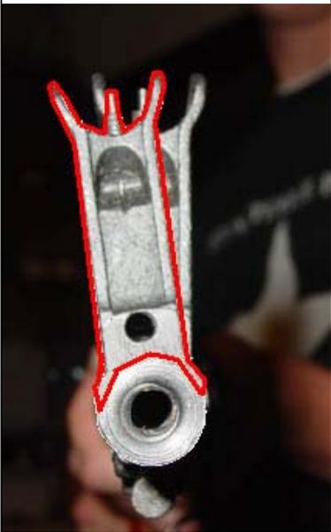
The second place Cant is common is on the gas tube. The picture to the left depicts looking at the rifle head on if the
