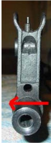
its right side with left side facing up, it's a good idea to get some one to hold the rifle, or if you have a vise, rap a towel around the rifle a secure it. Start taping on the pins with a little force, not to much at first. Slowly increase how hard you hit it until they start to come out.
