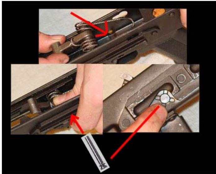
Place the hammer back in the rifle as shown with the hole lined up with the hammer axis pinhole on the receiver. Hold the hammer in place and reinsert the hammer axis pin, do this with the left side of the rifle facing up. The fat head part of the axis pin should keep the pin from falling all the way through the rifle; make sure the head of the axis pin is on the left side of the receiver. I recommend you take a piece of scotch tape and tape the pin in place until you finish installation.
