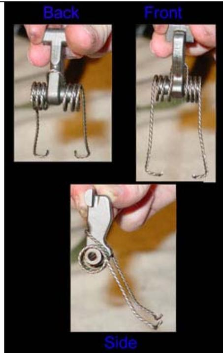
To reinstall, first wrap the hammer spring around the hammer as shown in the above picture.
