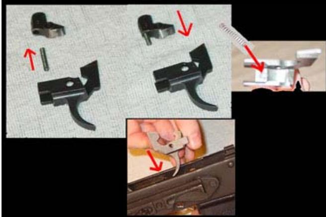
Next take the hammer and disconnecter and reassemble them as shown, make sure the disconnecter spring is in the hole inside the disconnecter and the small notch inside the trigger. Reinsert the trigger and disconnecter into the receiver as a single unit, make sure they do not separate because the spring inside the disconnecter will come out, and the two holes on the bottom of the trigger and disconnecter will not line up for the trigger axis pin.
