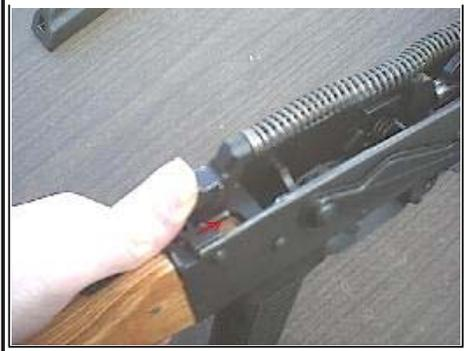
Now you can fully remove the recoil spring assembly.
