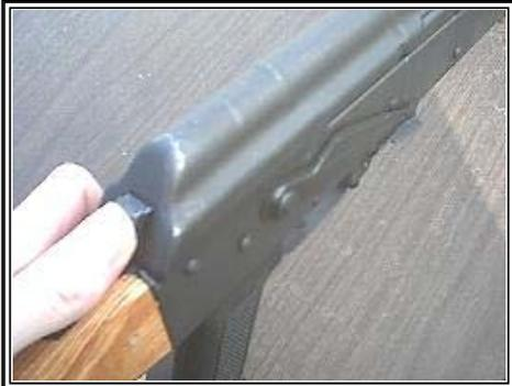
Now push the retaining tab forward until it clicks under the receiver cover.
