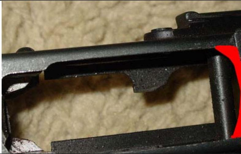
Next you need to clean up the rounded profile of the magazine well as highlighted in red in the above picture. Its best to take off a little at a time and test fit your drum/magazine. Once it fits fine take a file and smooth out the rough edges.
