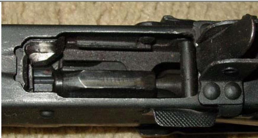
Once finished the well should look similar to above photo(note in this picture I did not smooth out the rough edges with a file yet which is the last step. Make sure you file down the rough edges and clean out all the metal shavings before shooting.
