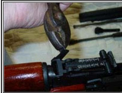
With the lever not quite vertical, grasp the rear end of the upper handguard/gas tube assembly and lift it up from the rear sight block. It might be necessary to wiggle the takedown lever back and forth to locate the release point for the rear end of the upper handguard/gas tube assembly. Once the rear end of the assembly is clear of the rear sight base, pull the front of the gas tube away from the gas block.
