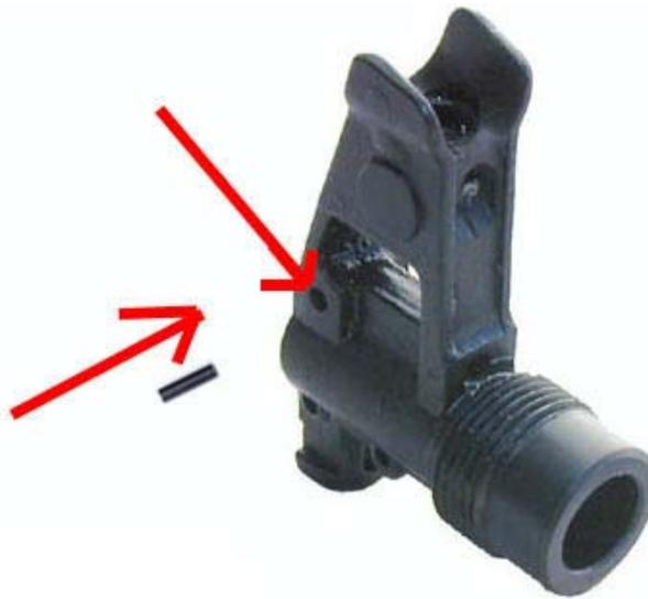
Now you need to flatten the ends of the pin out so you must place one side of the pin against a flat hard metal object and tap of the opposite side with a pin punch to get it to flatten out, when you are finished on one side switch sides and do the other. View the picture to get an idea of what it should look like.
