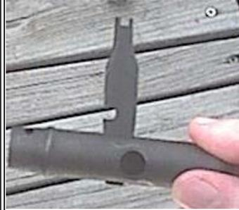
The next tool that can be assembled is the sight tool. This tool is used to adjust the elevation of the center sight peg in the front sight. Please view the Sighting in Your AK tutorial for instructions on how to use this tool. To assemble this tool stick the blade end of the multi tool through the large slot down through and out the small slot in the tool kit case.
