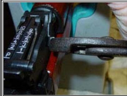
Using a pair of pliers or the bullet tip of a cartridge, rotate the takedown lever located on the right side of the rear sight base upwards.
